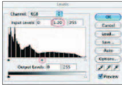
FIGURE 3-11. LEVELS GAMMA ADJUSTMENT. The midtone slider has been moved to the left to gamma value 1.20, lightening the midtones.
